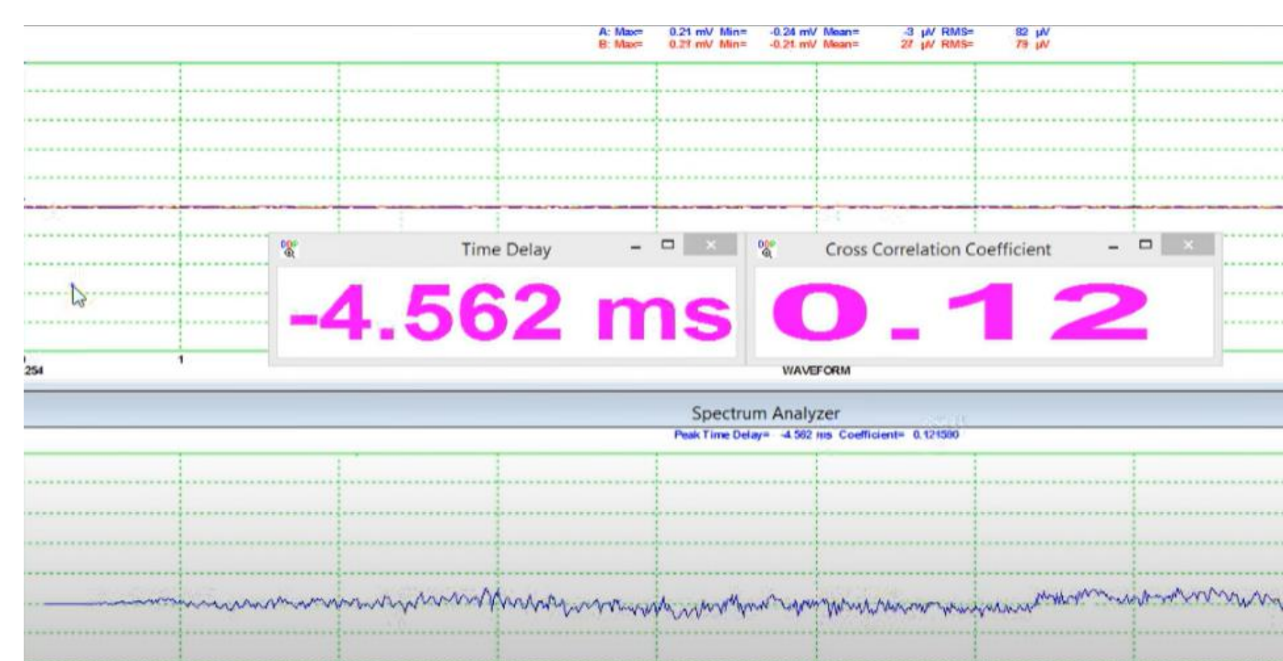
Using cross correlation to measure time delay and seeing the latency of the app.
