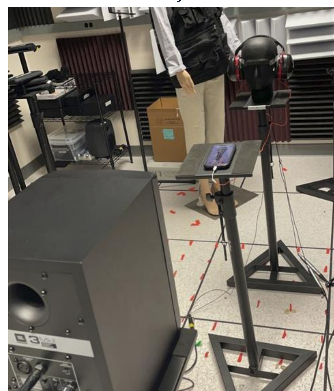
Testing the app using an Audio Interface, a head-replica with built in mics and measuring the audio signals by the external sound from the speaker and the sound coming out of the developed app.
